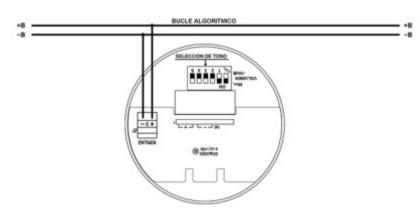
Before installing it is necessary to code the address that the siren will occupy within the algorithmic loop (see Equipment Coding).
